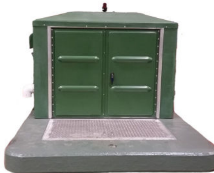
Sealed and gasketed weather-tight insulated fiberglass enclosure with a 3-point lock. The enclosure is gel-coated inside and out and mounted on a reinforced 8" concrete base. Multiple color options are available for exterior and base coatings. Aluminum bases are also an option for fiberglass wetwells.
