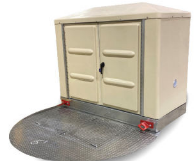
Sealed and gasketed weather-tight insulated fiberglass enclosure with a 3-point lock. The enclosure is gel-coated inside and out and mounted on a reinforced 8" concrete base. Multiple color options are available for exterior and base coatings. Aluminum bases are also an option for fiberglass wetwells.
